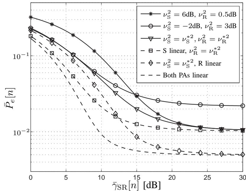
Fig. 5. Average bit error probability in terms of the first hop SNR when the second hop SNR  $\bar{\gamma}_{RD}[n] = 20\text{dB}$  and  $A_S = A_R = 1$ .
