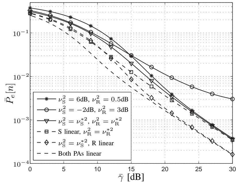
Fig. 4. Average bit error probability when  $\bar{\gamma}_{SR}[n] = \bar{\gamma}$ ,  $\bar{\gamma}_{RD}[n] = \bar{\gamma} + 5\text{dB}$  and  $A_S = A_R = 1$ .
