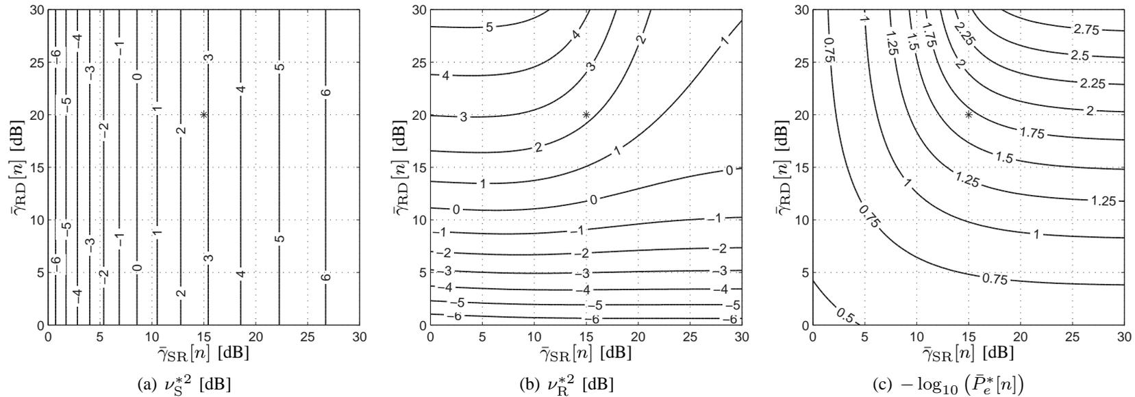
Fig. 3. Contour plots for the optimized input back-off factors and the minimal bit error probability when  $A_S = A_R = 1$ . The SNR pair  $(\tilde{\gamma}_{SR}[n], \tilde{\gamma}_{RD}[n])$  considered in Fig. 2 is marked with \*.
