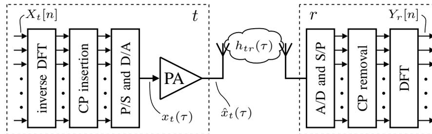
Signal model from transmitter  $t \in \{S, R\}$  to receiver  $r \in \{R, D\}$
