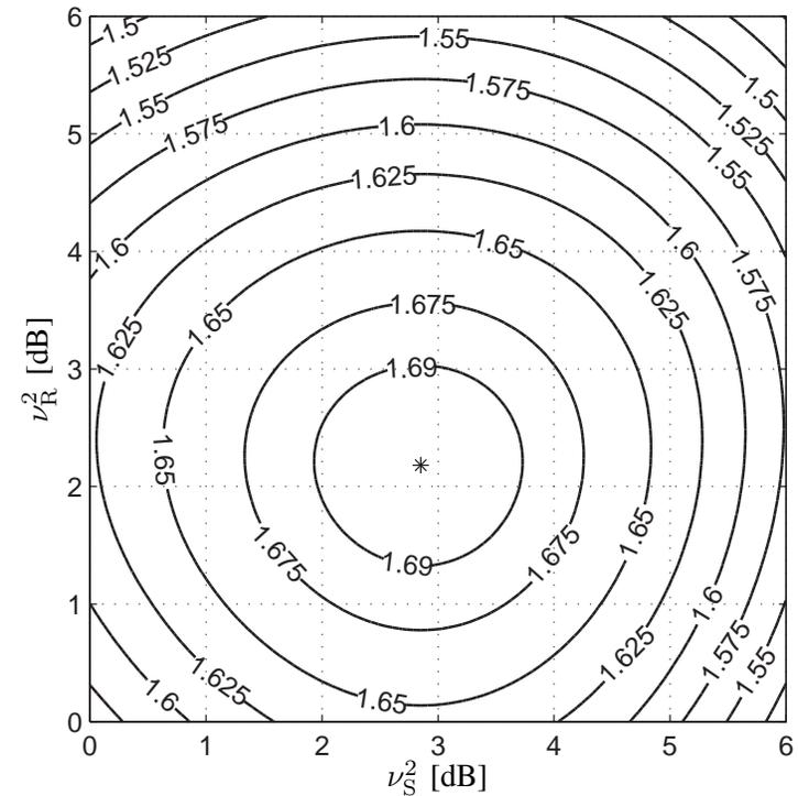
Fig. 2. Contour plot for  $-\log_{10}(\bar{P}_e[n])$  in terms of the input back-off factors when  $\bar{\gamma}_{SR}[n] = 15\text{dB}$ ,  $\bar{\gamma}_{RD}[n] = 20\text{dB}$ , and  $A_S = A_R = 1$ . The minimal bit error probability  $\bar{P}_e^*[n] = 2.0 \cdot 10^{-2}$  is reached with  $\nu_S^{*2} = 2.85\text{dB}$  and  $\nu_R^{*2} = 2.18\text{dB}$  (marked with \*).
