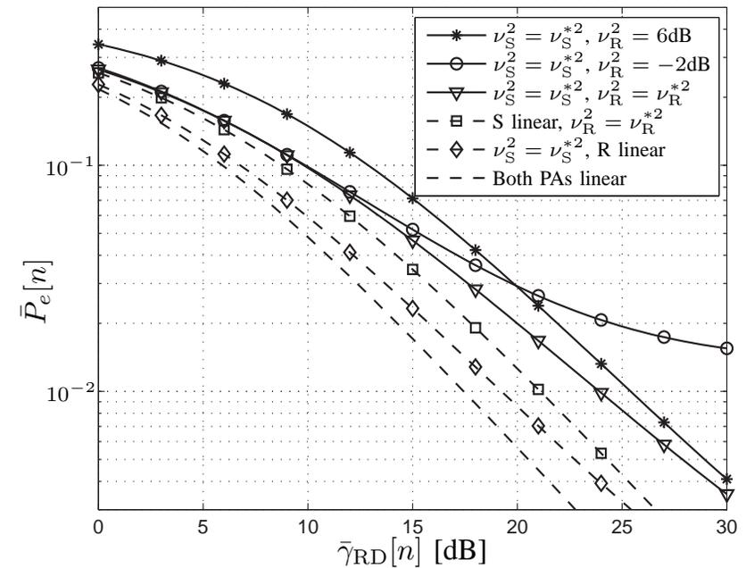
Fig. 6. Average bit error probability in terms of the second hop SNR when the first hop SNR  $\bar{\gamma}_{SR}[n] = 15\text{dB}$  (hence  $\nu_S^{*2} = 2.85\text{dB}$ ) and  $A_S = A_R = 1$ .
